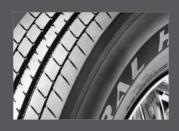
Scruff ribs protect sidewall from curbing and cutting.
